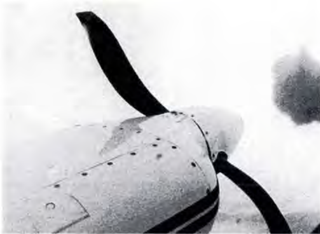
The pilot's first indication of trouble was a terrible vibration from the left engine. As the propeller came to a stop and folded back toward the nacelle, he thought he had hit another aircraft.
